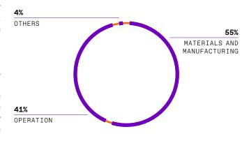
Figures in this chart are based on the EPD published for the most representative configuration of our low-rise elevator installed in Europe. Most of this elevator's GHG emissions over the course of its life cycle are related to the use of materials, manufacturing and operation. Their relative importance is strongly influenced by the elevator's configuration and where it is installed.
