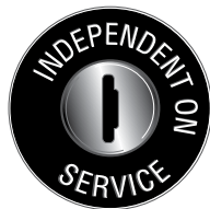
Independent service keyswitch Elevator no longer responds to hall calls and remains on a floor with its doors open until a floor is selected and the "Door Close" button is held; then, the elevator starts to travel. Useful when transporting large goods or moving groups of people between certain floors.
