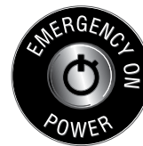
Emergency power keyswitch Provides in-car control over the elevator. When the keyswitch is in the "ON" position, the elevator will be controlled by the attendant and will not respond to hall requests. The keyswitch, when in the "ON" position, will be overridden by emergency operations (fire service, emergency stop, etc.).
