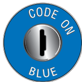
Code blue keyswitch Mounted in hall station to call the car to the respective floor in an emergency.
