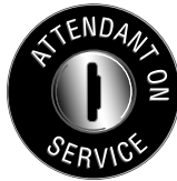
Attendant service keyswitch Provides in-car control over the elevator. When the keyswitch is in the "ON" position, the elevator will be controlled by the attendant and will not respond to hall requests. The keyswitch, when in the "ON" position, will be overridden by emergency operations (fire service, emergency stop, etc.).
